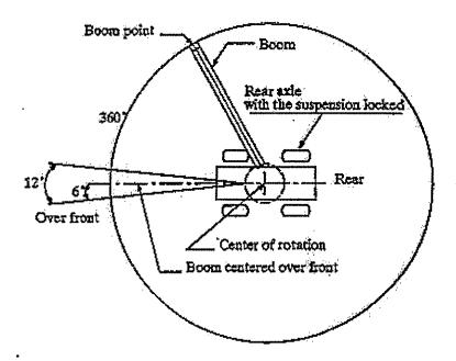
Crane lifting capacities on tires depend on tire capacity, condition of the tires and tire air pressure. Tires must be inflated to the recommended pressure before lifting. (See operator's manual.) The recommended pressures are indicated either in the cab or next to the wheels. When handling loads in the structural range with the capacities close to maximum ratings, travel should be to 'Creep Speed'. 2.5 MPH (4 Km/HR) capacities are permissible on main boom only. NOT on boom extension.
