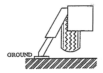
When lifting on outriggers, extended outrigger rated lifting capacities, section 1, will only apply if outriggers are fully extended. Tires must be clear off the ground.
